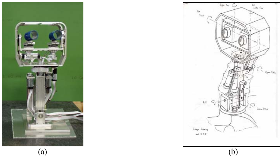
Figure 12: Picture of the anthropomorphic head and DOF disposition.
