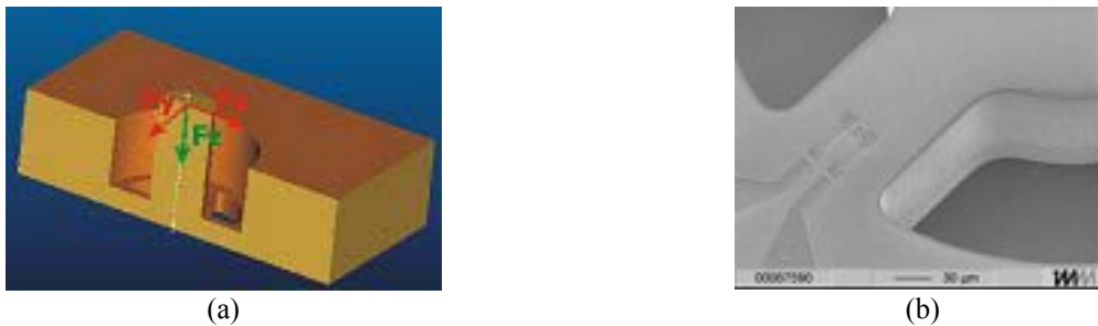
Figure 9: Section of the sensor: 3D model (a) and SEM picture of implanted piezoresistors in one tether of the membrane (b).
