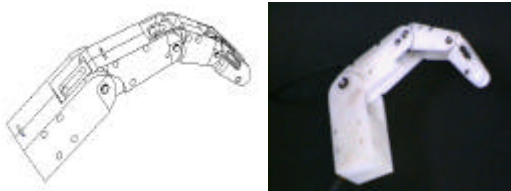
Fig. 3: General drawing and the first prototype of the finger
